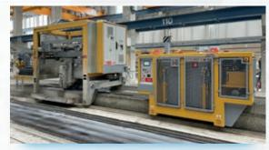
**ELEMENT CUTTING** Automatic multi-angle Saw with Counterweight Trolley
