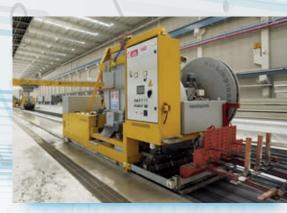
CLEANING-OILING-WIRE PULLING Automatic multi-function vacuum Bed Cleaner
