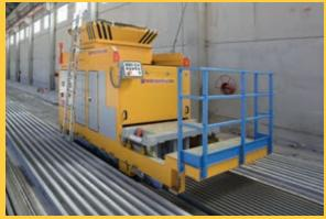
Element casting, Wet Casting WF
