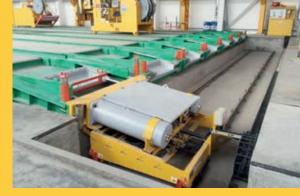
Stressing and detensioning of the steel wires
