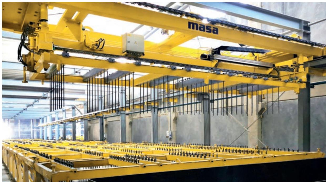
Placement of reinforcement elements
