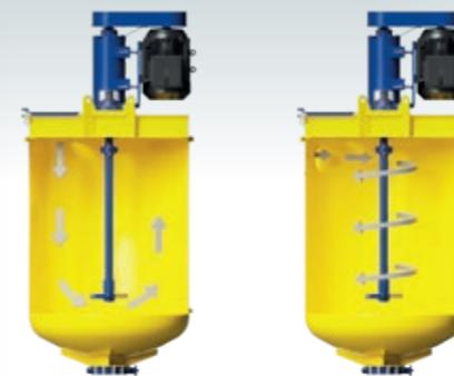
Schematic diagram: Different flow directions at vertical (l.) or tangential (r.) feeding of the liquid components.
